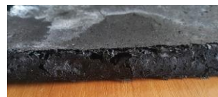
Fig. 5. Defective PVC board
