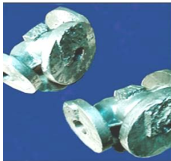
Fig.5 Cast blanks for a high-strength corrosion-resistant 05Kh22AG15N8MFL (0.05C21CrN15Mn8NiV) steel regulator: R_{p0.2} = 400 MPa; R_m = 680 MPa; A_5 = 37\% ; RA = 50\% ; KCV-70 = 1.8 MJ/m 2 ;
