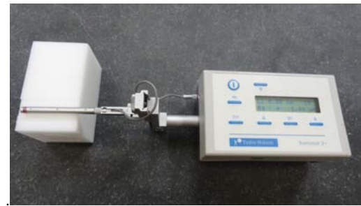
Fig. 7 Surface roughness measurement using roughness meter Surtronic3+
