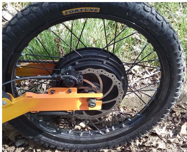
Fig. 5 Rim-integrated BLDC motor.
