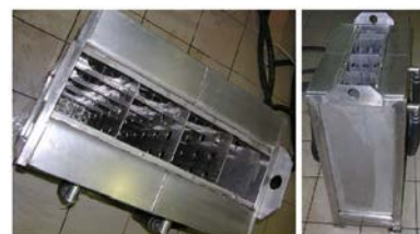
Fig. 14. NO-145 decontamination unit used for solid radioactive waste tests at the Beloyarsk NPP
