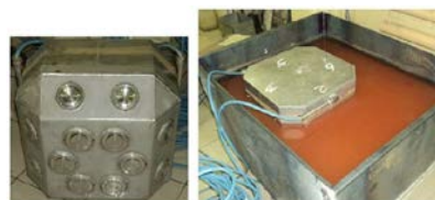
Fig. 23. Ultrasonic decontamination of fluid radioactive waste storages
