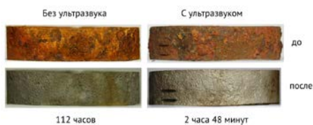
Fig. 16. Solid radioactive waste fragments before (top) and after decontamination (bottom) using conventional technologies (left) for 112 h and ultrasonic treatment (right) for 2.8 h
