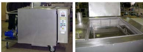
Fig. 18. MO-128 decontamination unit in the All-Russian Research Institute for Inorganic Materials
