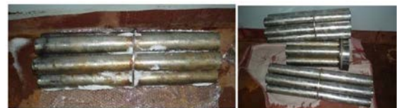
Fig. 13. Fragments of irradiated fuel assembly shrouds before (left) and after decontamination (right)
