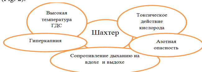
Fig.2. The main factors of adverse effects on a human induced by the mine self-rescuer.
