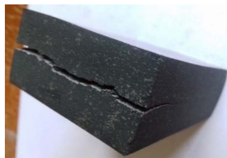
Fig. 1. Common view of the billet after compression more than 10 % during the rolling process
