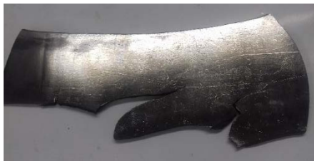
Fig 3. Common view of the billet after compression more than 10 % during hot rolling at 1100 °C
