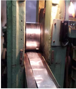
Fig. 7. Rolling unit Mill DUO-280 (Rubin company, Kharkov)
