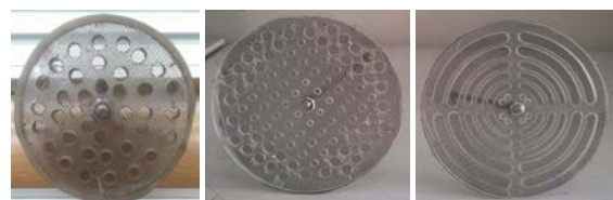
Fig. 5. Different hole types in porous plate (hole diameter 2-5mm).
