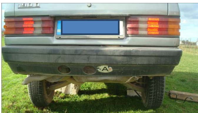
Figure 2. Preparing the passenger car Mercedes 190 D for vibrations measurement at the rear axle assembly
