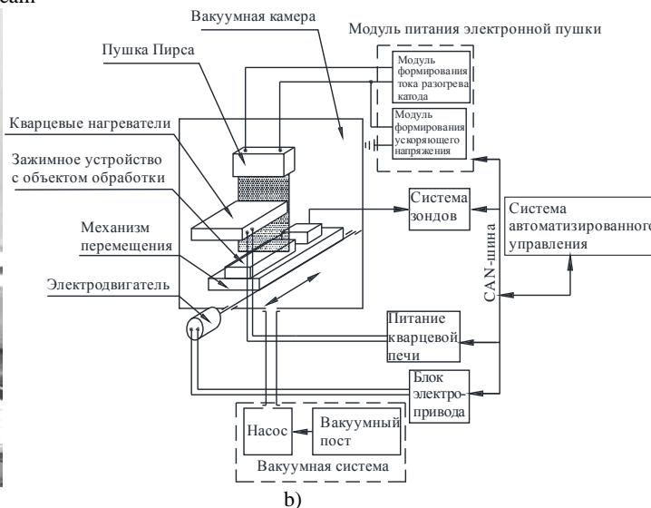
Fig. 1. Appearance (a) and schema (b) installations for the finishing electron-beam processing of optical elements, which improves the physical-mechanical properties of their surface layers: 1 – vacuum gauge magnetic locking VMB-8 (ВМБ-8); 2 – gauge ionized-thermocouple VIT-3(ВИТ-3); 3 – vacuum chamber; 4-electric mechanism of transfer mechanism of optical elements; 5 – PC control; 6 – modules of temperature measurement in the treatment area and sensing electronic flow; 7 – thermal management system of optical elements based on device RIF-101 (РИФ-101); 8 – central unit of automatic control system; 9 – power supply and control system of electronic gun of Pierce; 10 – electric motor control.
