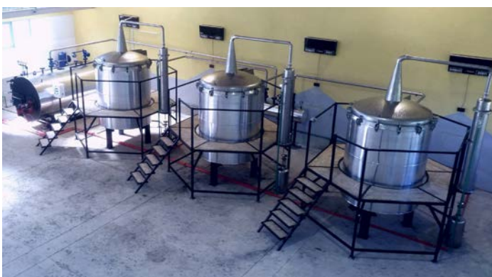
Fig. 6 Complete equipment for essential oil distillation with new solution of the substance flow system (produced by "Solar mont" Ltd, Gradiska, B&H)
