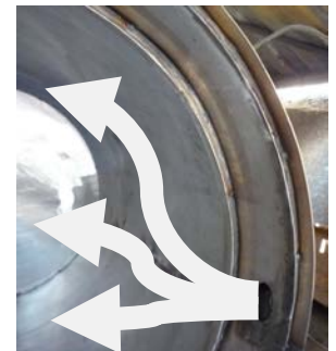
Fig. 2 Supply of steam on top of the distiller - new solution of distiller
