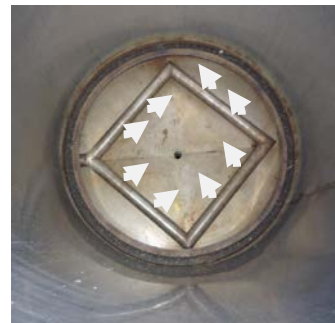
Fig. 1 Injection of steam from the bottom - typical distiller
