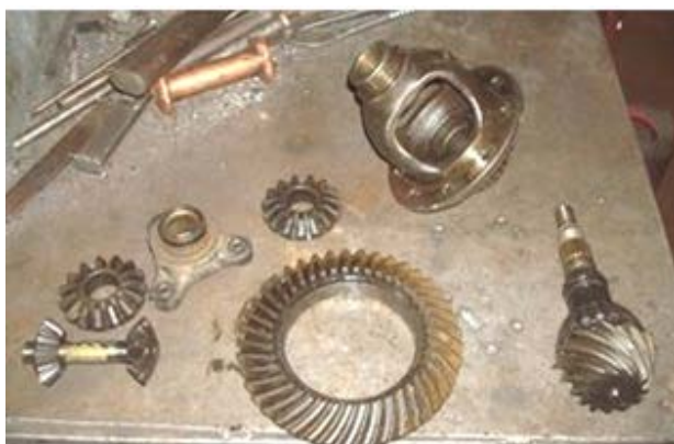
Figure 10. Condition of components of rear axle after disassembling
