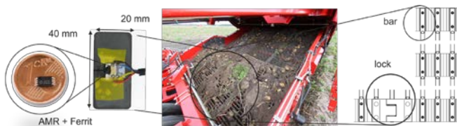
Fig. 5: AMR-Sensor (left [23]), conveyor belt (middle [24]), schematically (right)
