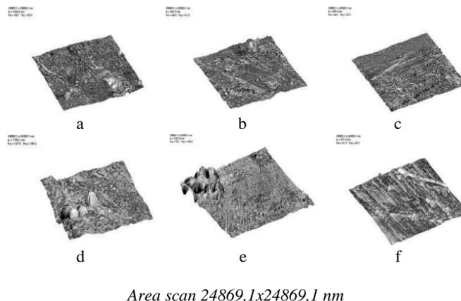
**Fig. 1** The surface morphology of film samples LDPE (a, d), PP (b, e), PET (c, f) the source (a, b, c), treated with pulsed laser light with a 2.0 W/cm<sup>2</sup> power density (d, e, f)
