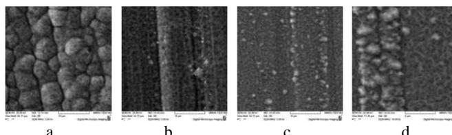
a - the initial coating, b - concentration solution FCO in the electrolyte 3% wt%, c - FCO concentration in the electrolyte solution 7 wt%, d - concentration particles of polytetrafluoroethylene obtained by dispersing the laser, 0.1% wt%
