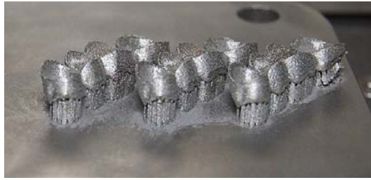
Fig. 1. SLM of dental bridges
