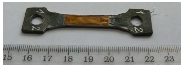
Fig. 3. Cast tensile test specimen with strain gauge.
